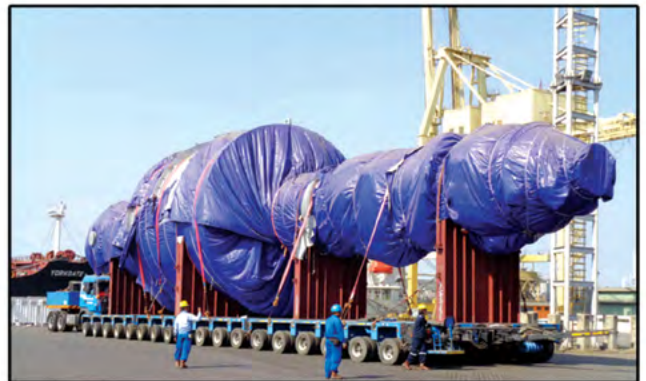
REACTOR Transportation (L X W X H @ 35.0 X 7.95 X 8.45 M)
