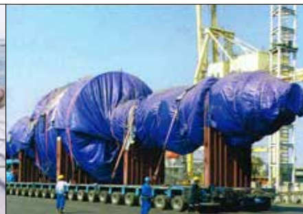
REACTOR Transportation (LxWxH @ 35.0X7.95X8.45 M)
